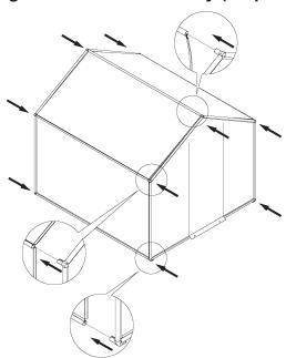
12. Line up the Connectors on the Front and Rear Panels and connect to the Body Panel (M). The uppermost pole in the Body Panel should be turned with the connection downward. All other poles should be turned with the connection upward, as shown.
